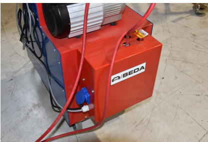
Optional oil separator for pure refrigerant recovery
