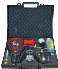
The top model among cooling system testing devices. In addition to pressurization using a hand pump or compressed air, pressure can also be built up by heating the engine. This allows for testing the cooling system pressure, cylinder head tightness, and the fan in a single operation once the operating temperature is reached.
