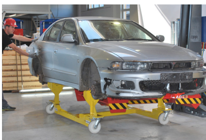
Forklift free loading with trolley
