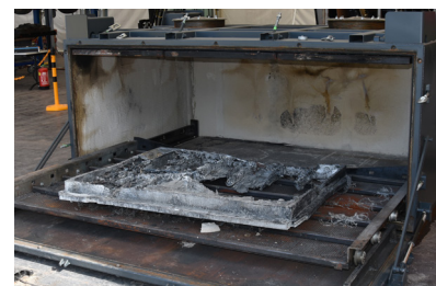
HV BAT-Box with burnt-out car battery after testing
