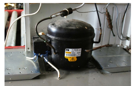
Compressor secured in clamping area
