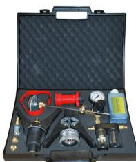
The top model among cooling system testing devices. In addition to pressurization using a hand pump or compressed air, pressure can also be built up by heating the engine. This allows for testing the cooling system pressure, cylinder head tightness, and the fan in a single operation once the operating temperature is reached.
