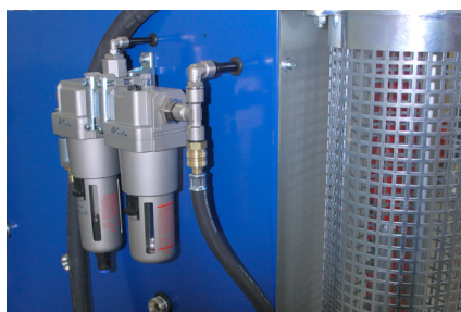
Air processing unit (left) with fuel quality control (right)
