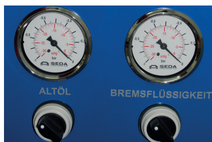
Vacuum gauge and switches
