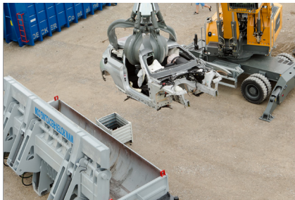
Loading the press with a separate crane
