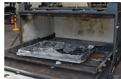
HV BAT-Box with burnt-out car battery after testing
