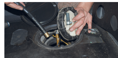
Higher suction rate by dismantling the fuel pump on the tank and the hose leading directly into the tank.
