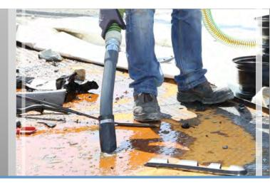
The FS-216 fluid and oil sludge cleaner is the perfect solution for the extraction of liquids with dirt or metal particles from the floor, catchment areas or bins.
