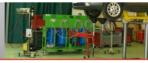
The 4-Fluid Station is a compact and mobile entry-level solution for smaller dismantlers with a de-pollution rate of up to 5 vehicles per day.
