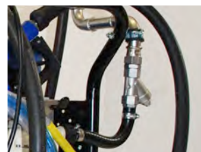
Stainless steel in-line filters: Sieve to be cleaned weekly
