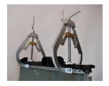
"The SEDA Radiator Tension Clamps set is universally applicable and easy to apply. When used properly the danger of incorrect installation of the water tank and possible consequences (leakness) can be reduced to a minimum."
