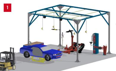
Lift vehicle with forklift on the trolley
