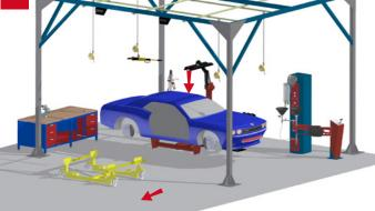
Fix to secure the vehicle by the hydraulic roofclamp, remove trolley, dismantle the wheels and exterior parts and prepare for the drainage
