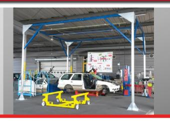
Efficiency, safety and ergonomics are keywords in todays recycling companies. For this reason, SEDA has developed an All-In-One Solution together with car manufacturers and dismantlers. This solution is the first complete system for ELV de-pollution and dismantling which now can be performed on a new special TiltLift by one person independently.
